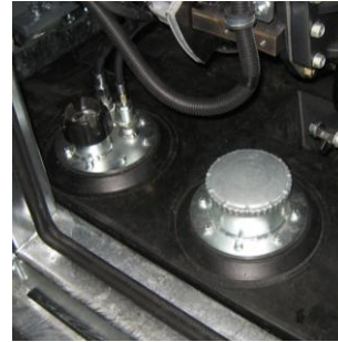
Fuel tank Fully bunded, corrosion-free, 300 liter, high-density polyethylene (HDPE) fuel tank, located in base of canopy.
