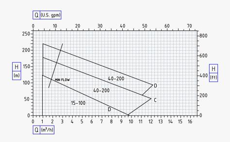
» Alloy Double Stage Turbine Pump 3500 rpm 60hz
