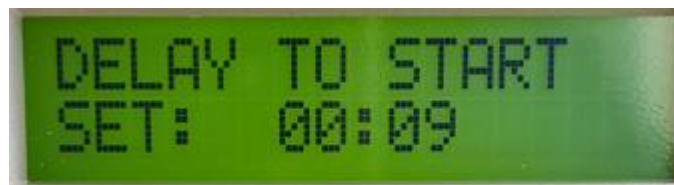
Fig.8. Delay to start panel
