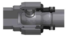
**Cardan Joint**: Cardan joint is the best solution for heavy application with high speed rotation and high pressure inside the pump casing. It improves the allowable torque up to 4 times torque with the same pump size. It is available with internal metal joint protection to for an additional improvement of the rubber service life.
